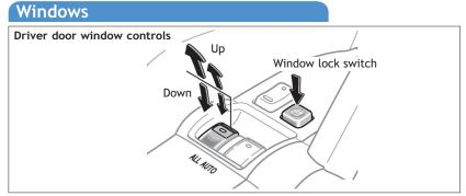
Automatic operation (all windows) Push the switch completely down or pull it completely up and release to fully open or close. To stop window midway, lightly push the switch in the opposite direction.
